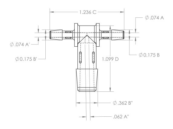
ANTI-ROTATION DEVICE 4 PLACES PER BARB NO MOLD PARTINGLINE PERMITED ON CONICAL SURFACES ALL DIMENSIONS TYPICAL MATERIAL-316SS VIEW SHOWN LOGO SIDE UP 'A' CAVITY DESIGNATED BY A SMALL DOT ON BARB NECK
